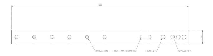
All dimensions are in mm; tolerances according to ISO 2768 m-H
